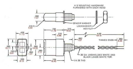
**DUMMY HEADS** Used to provide a tape support surface in applications where all positions of the head nest are not used. Same face finish and contour as regular heads. Supplied in standard mount configurations.
